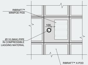
Use of Xpod<sup>®</sup> Mini Pods to create zone for pipes to penetrate slab.
