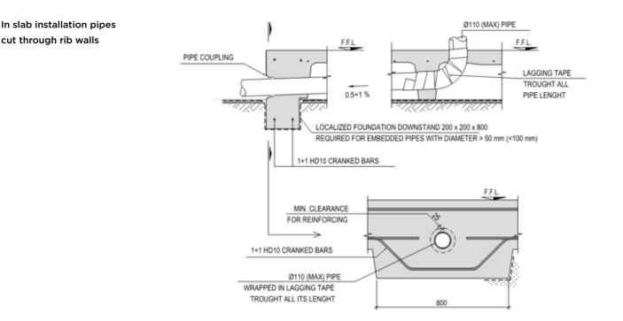
Use of Xpod<sup>®</sup> Mini Pods to create zone for pipes to run without compromising the ribs
