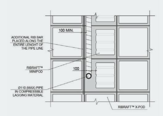
Typical drop down detail for sewer line to prevent it being visible at exterior of slab
