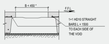
(\*) IF B > 450 mm PLACE 2 HD10 CRACK CONTROL BARS @ 200 L = 2000 AT EACH CORNER OF THE PENETRATION
